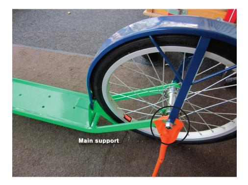
Main support is "inside", Then the fender support, Kickstand is on the outside closest to the nut.
