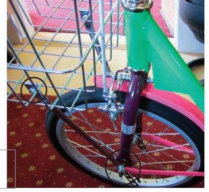
Wheel goes on forks first, Then the fender supports, Then the basket supports
