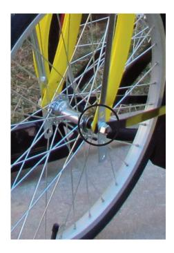
To tighten wheel nuts Use a wrench on both the inner nut and outer nut
